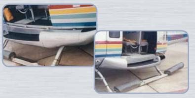
The Extended Passenger Step is identical in profile and appearance to the External Auxiliary Fuel System, with the obvious exception that the step portion is lengthened to provide greater step area. Aft of the step is a small items storage locker and available area for mounting side-facing flood lights to illuminate the area surrounding the aircraft for such tasks as emergency medical evacuation scene work.
