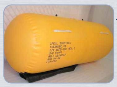
Six floats (2 forward, 2 middle and 2 Aft) are used on the Bell 412. The right and left forward and middle floats
