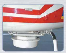
Our Universal Pod Bracket installs on the Bell 206 Series by utilizing the rotorcraft's existing Cargo Hook Provisions. This Bracket allows for the installation of a Microwave Antenna Pod in order to permit live video downlinks from the helicopter.
