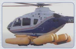
Each kit includes four floats. Each float is constructed utilizing lightweight urethane-coated nylon fabric. Each float has inlet check valves
