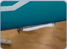
The Rear Utility Mount allows for the installation of a searchlight, camera gimbal or other optional equipment on the Bell 206 & 407 on the lower Aft belly, Aft of the baggage compartment at the rear of the jack-point / tie-down position. This configuration frees the nose area for installation of other equipment and provides additional ground clearance.
