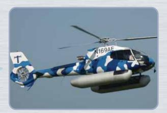
Apical is the holder of 30 Float and Float/Liferaft Systems STCs for the following helicopter models:
