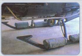
The Step Assembly is designed to provide aircrew and passenger access to the helicopter cockpit or cabin. The step supplements the OEM skid toe mounted step and includes a non-skid surface. The Step Assembly is constructed of high quality aluminum which has been anodized to protect it against corrosion. The Step Assembly is mounted high enough that it may be used with any Apical float configuration (Tri Bag Emergency Floats, Single Bag Emergency Floats). The Step Assembly contains the following:
